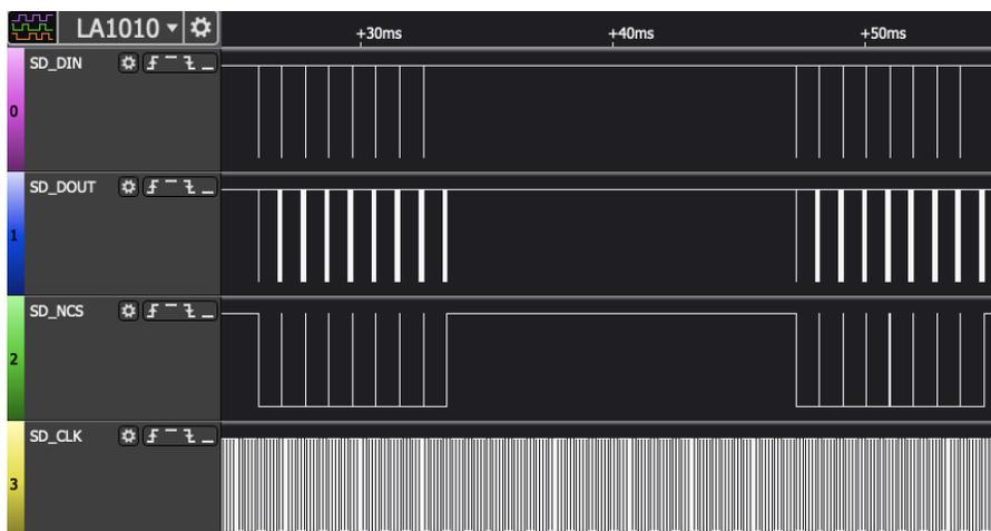
Fig. 4. SD signals on a logic analyzer
